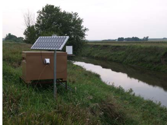
fig 11. Event triggered composite sampler at site 50
