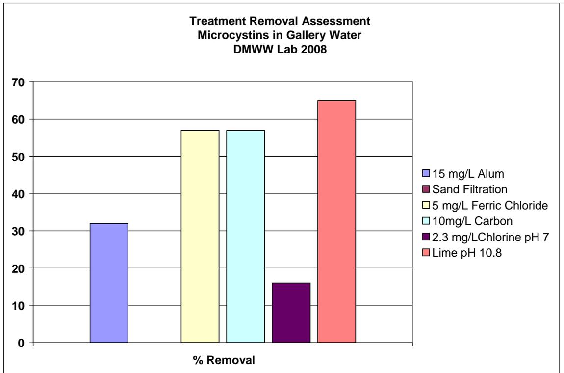
Figure 9. Microcystin Coagulant Removal Assessment
