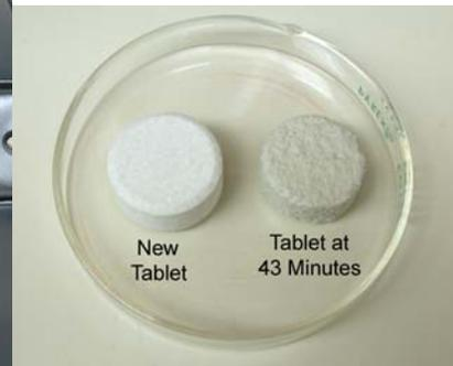
This study indicates if chlorine tablets were dropped into an ASR well, that they would reach the bottom largely intact. They would dissolve creating a zone of concentrated chlorine that would likely diffuse horizontally more than vertically.
